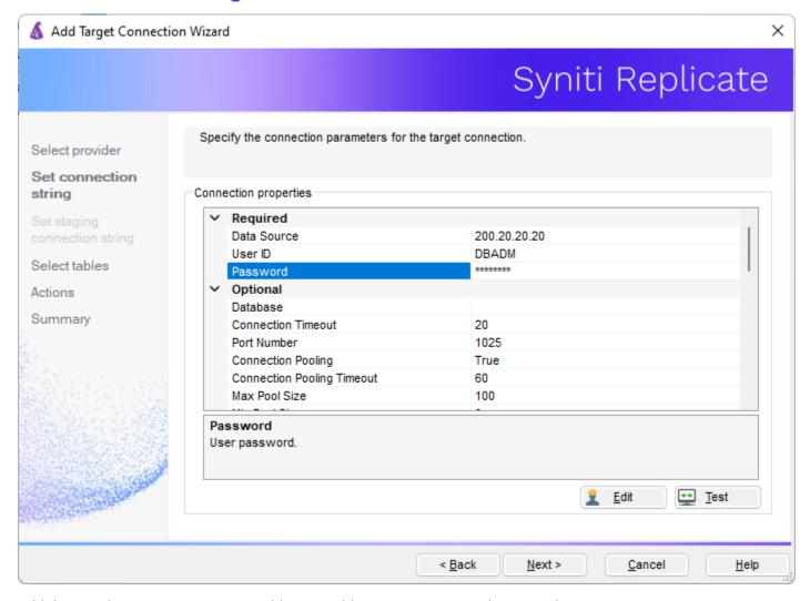
Add the Teradata server name or IP Address in addition to a user ID and password.
