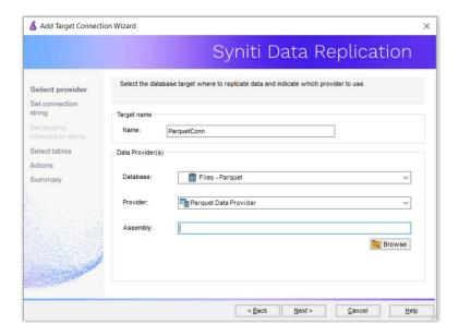
4. In the **Set Connection String** page, set a directory path for the output from replications between the source relational database and the Parquet file target.
